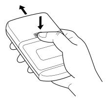
**2** Replacing the battery
